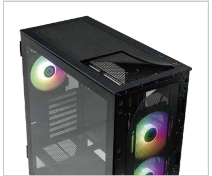
Magnetic Dust Filter on Both Top and Front Side
