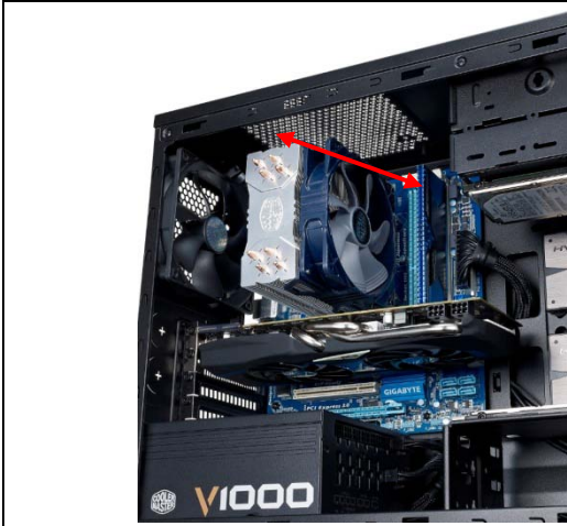
Supports air cooling, height up to 160mm
