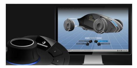
The On-screen Display1 provides a convenient visual reminder of the commands assigned to the Intelligent Function Keys, on your computer screen, enabling you to stay focused.
